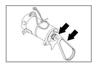
8. Slip the new drive belt into position. Push the rest of the drive belt up toward the motor belt pulley. Slip the drive belt over the motor belt pulley.
