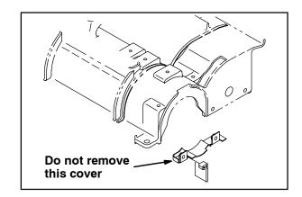
Using the M8 hex screw located under the brush motor, tension the **new** belt by applying 1.37 – 1.48 kg (3.01 – 3.26 lb) of force per belt at the middle of the span that is opposite the belt travel with a deflection of 0.10 inch.
