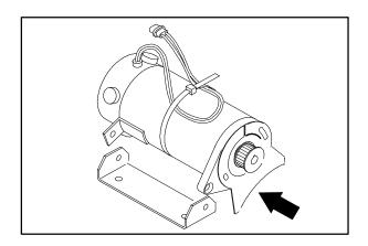
12. Tighten the drive motor pivot bolts to 18 - 24 Nm (15 - 20 ft lb). Re-check the belt tension.
