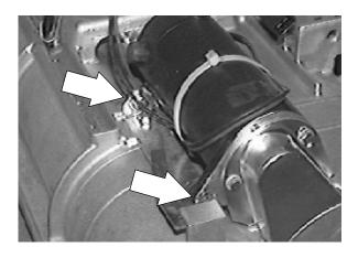
4. Remove the two M6 hex screws holding the belt cover on the motor that the belt needs changing. Remove the belt cover from the scrub head.
