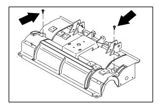
10. Tighten the two pivot bolts to 18 - 24 Nm (15 - 20 ft lb). Re-check the belt tension.
