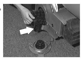
13. Reinstall the front cover using the four M8 hex screws. Tighten to 18 - 24 Nm (15 - 20 ft lb).
