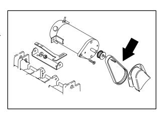
8. Slip the new drive belt past the lower belt cover and over the cogged pulley. Push the rest of the belt up to the drive motor and onto the drive pulley. Reinstall the rubber seal on the bottom drive pulley.
