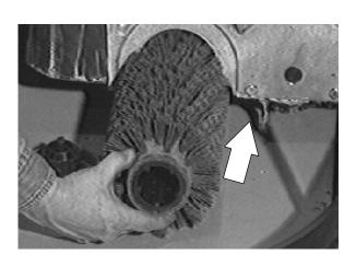
15. Operate the machine and check the scrub brushes for proper operation.
