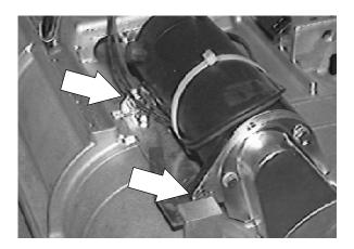
Reinstall the belt cover, two M6 hex screws, and washers. Tighten to 11 - 14 Nm (7 - 10 ft lb).
